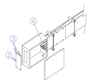
c) Unscrew four screws (3) and remove plate (2) (when the plate is installed).
