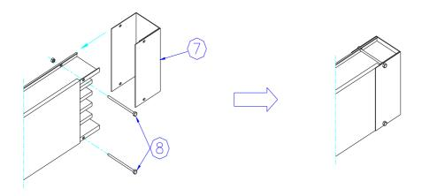
g) Fix the end cap (7) and tight the four screws (8).
