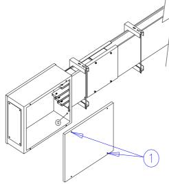
b) Unscrew four screws (1) and remove the lid.
