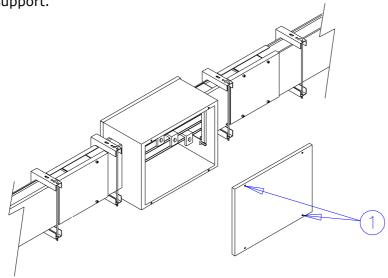
b) Unscrew four screws (1) and remove the lid.
