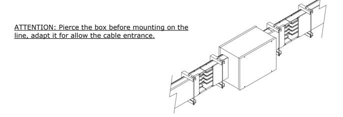
a) Fix the hanger and mount the center feed unit to two busbar elements as explained into "Assembly instruction line and GDA joint part; we suggest to support the center feed unit box with another support.
