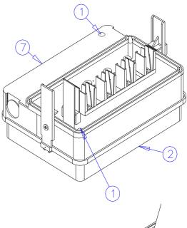
e) Insert tap off box in tap off unit positioned on straight element (10). Check that electrical grounding contact PE, is well done.
