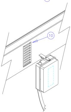
f) Bring near the two hooks (5) to straight element edge and block with screws (9) to the tap off unit body (7).
