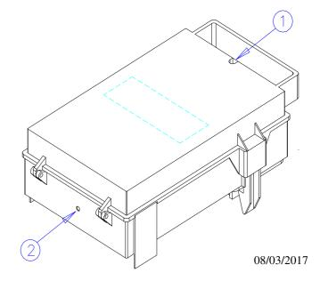
b) Mill the tap off body with a proper tool (max. diameter 48mm) in accordance to the selected cable. The correct hole execution is made easier by the dead hole (2) present on the hinge side.
