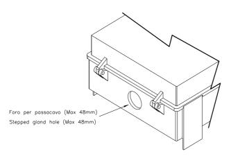
c) Insert the stepped gland, then insert cable and carry out all electrical connections. Check that the internal tap off box must be clean and check that there is not copper filaments or other conductive objects.
