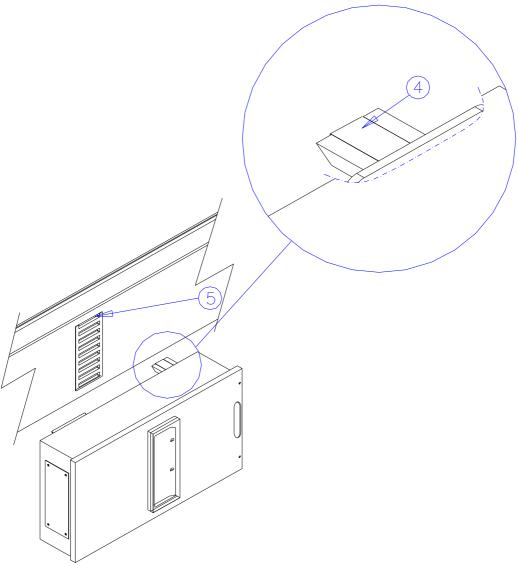
Rev.01 08/03/2017 e) Push in the tap off box and hook up the hooks to the bus duct (6) and thighten the screws.
